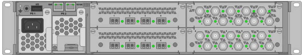
Figure 2. Cisco DCM Series D9900 MPEG Processor Rear Panel with AC and DC power supplies, 2 GbE cards, 1 ASI card and 1 ASI SFN card
